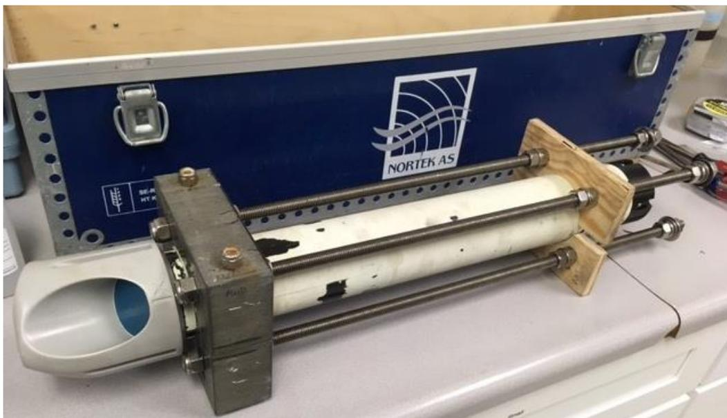
Figure 1.2.5: The 2 MHz Nortek ADCP with rigid mount for deployment from the R/V Benthic Cat.
