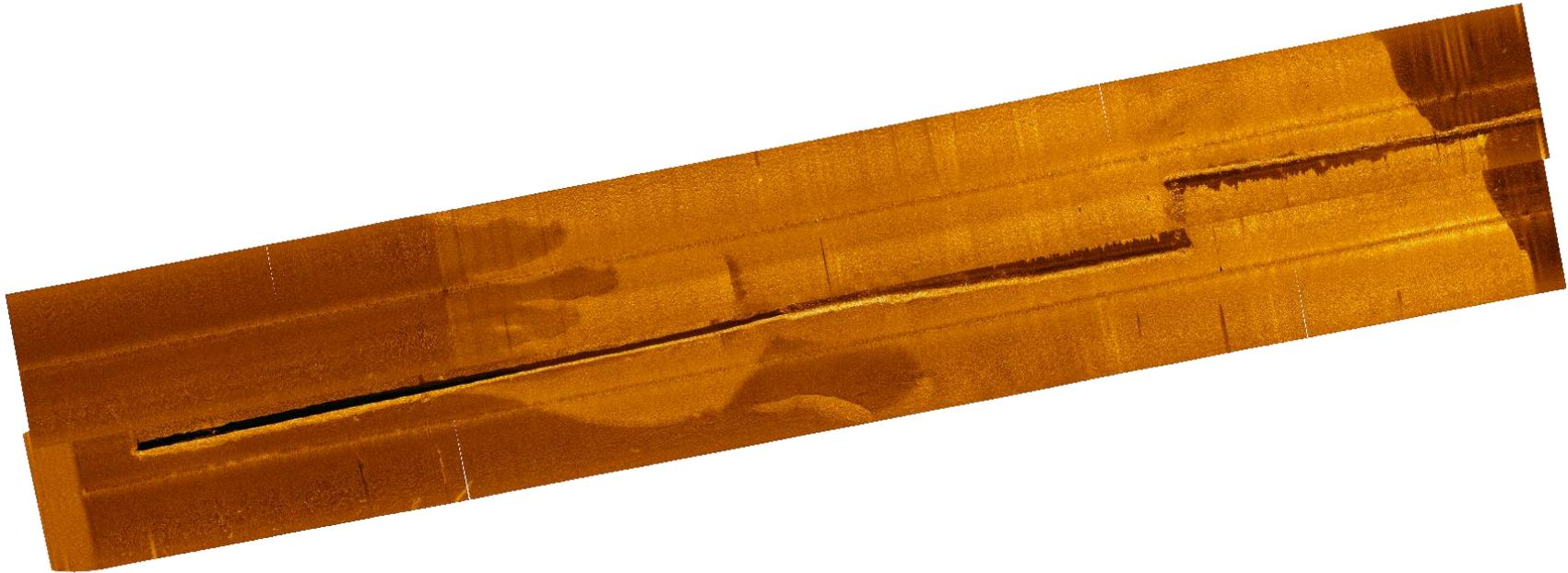
Figure 3.2.2: Side-scan sonar survey of SEOO used to obtain precision coordinates along the length of the pipeline and diffuser
