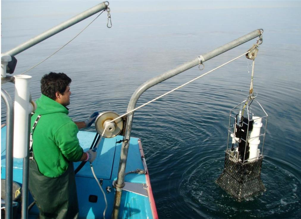
Figure 1.2.4: Sea-Bird SBE 19plusV2 CTD and typical shipboard casting equipment
