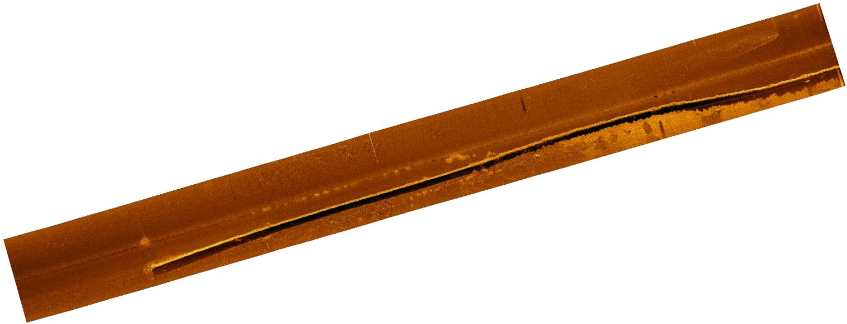
Figure 2.2.2: Side-scan sonar survey image of EOO used to obtain precision geo-referenced coordinates along the length of the pipeline and diffuser.
