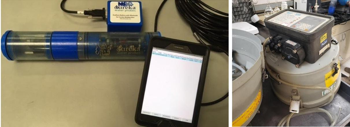
Figure 1.2.7: Eureka Handheld fDOM Probe with iPad data recorder for onshore sampling of the treated wastewater effluent prior to discharge and typical autosampler provided by EWA.
